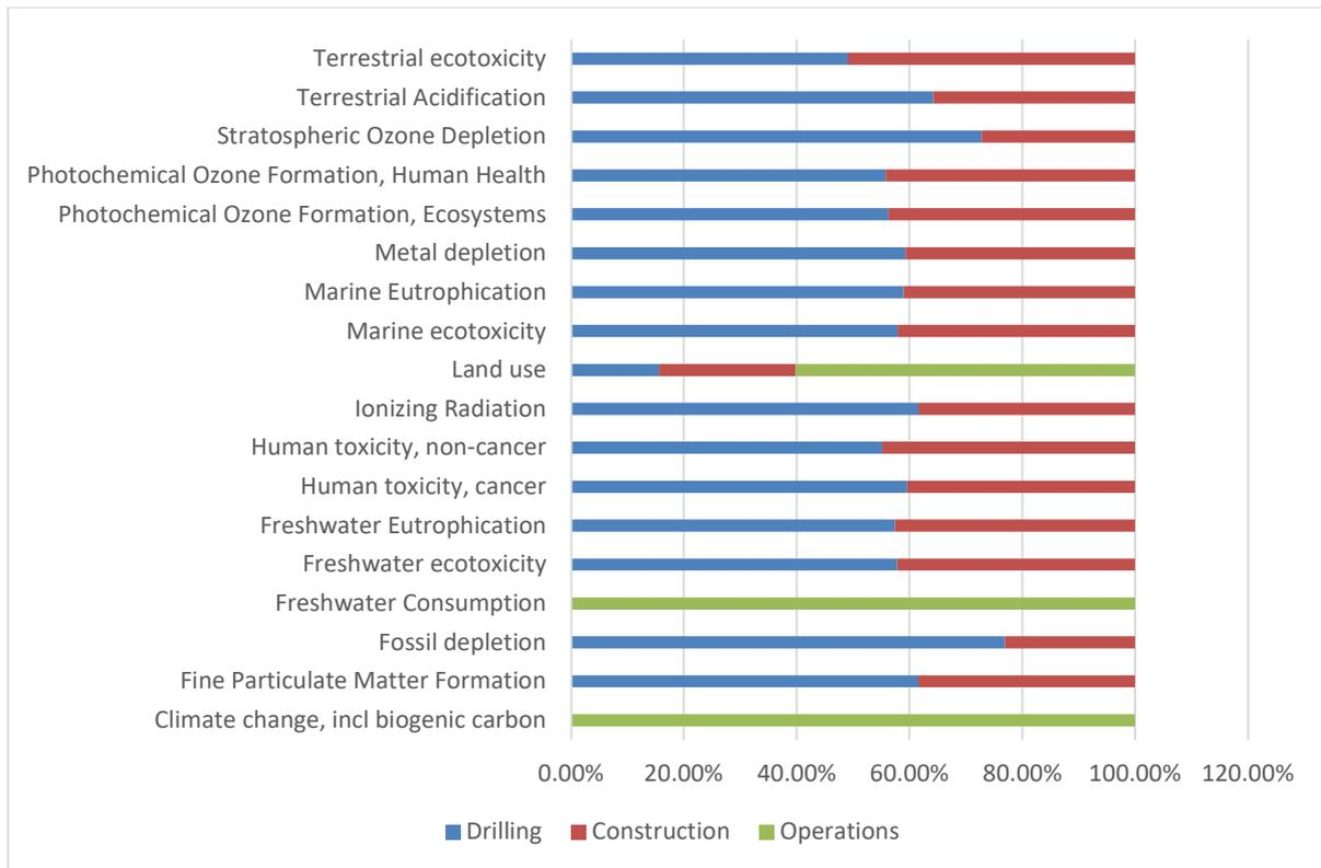
**Figure 15 Phase contribution to impact categories in the single flash plant**
