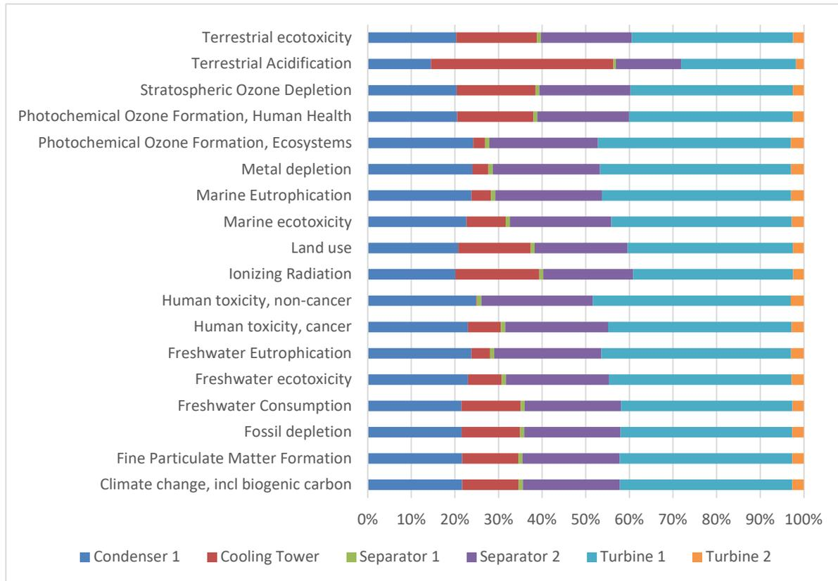
**Figure 18 Double flash plant component environmental impact contribution**
