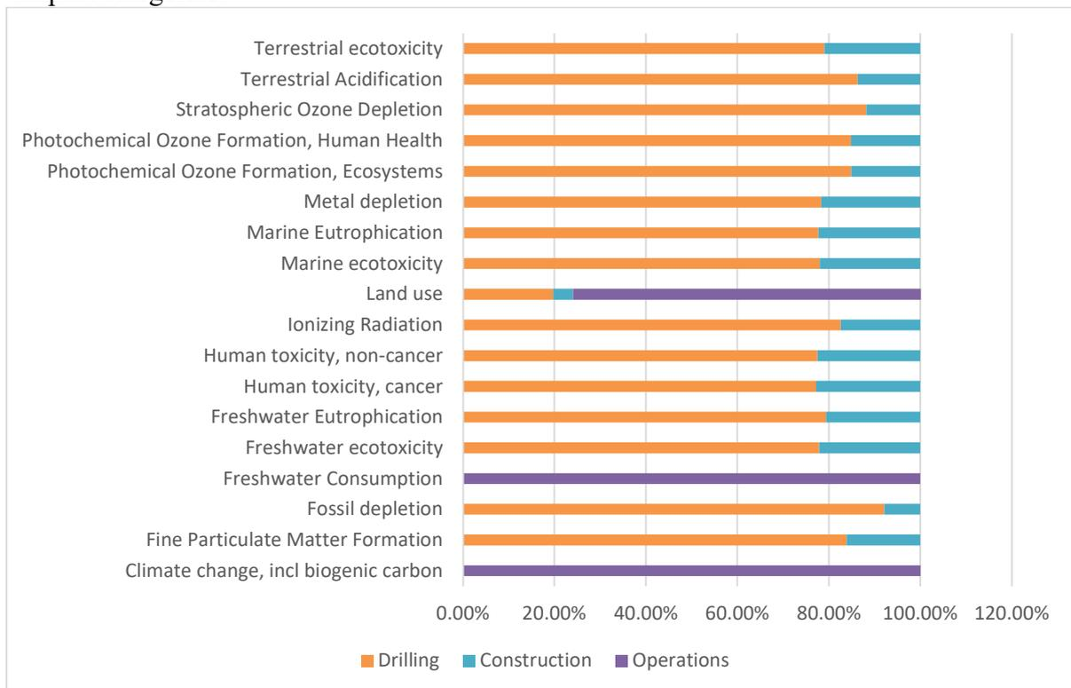
**Figure 16 Phase contribution to impact categories in the double flash plant**
