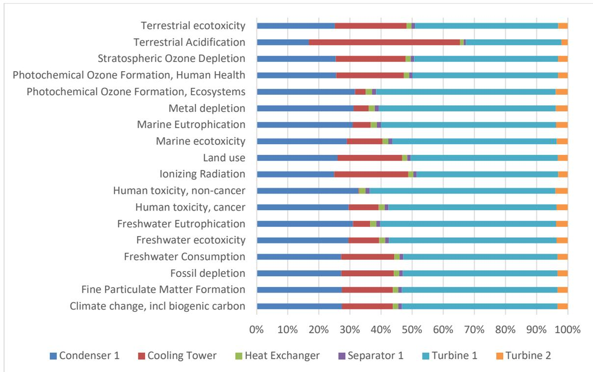
**Figure 19 Flash-binary plant component environmental impact contribution**
