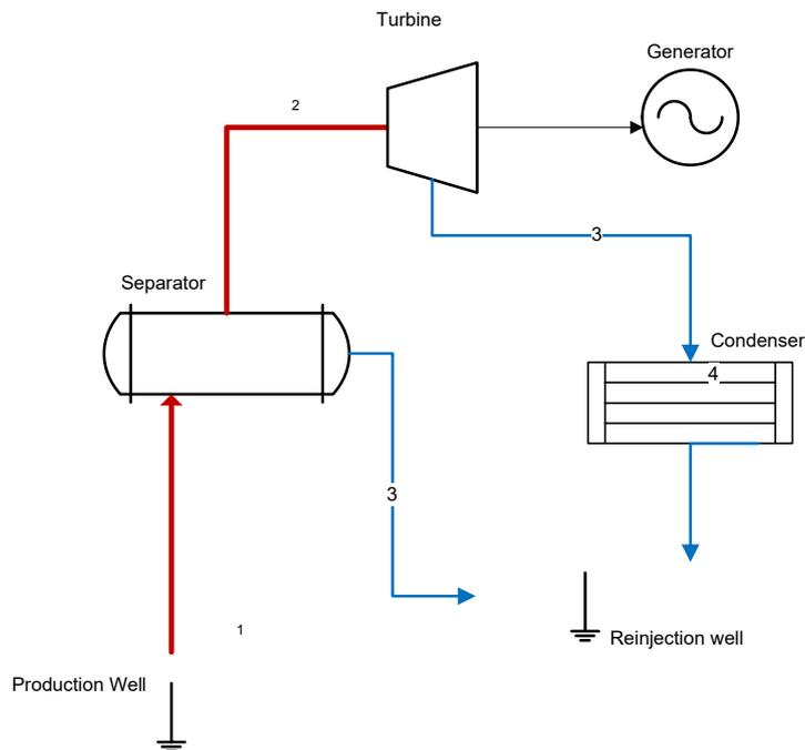
**Figure 2 Geothermal modular plant layout**
