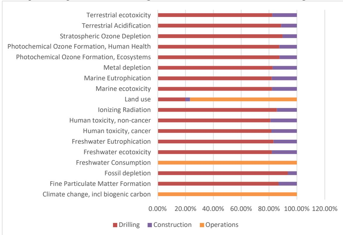
**Figure 17 Phase contribution to impact categories in the flash-binary plant**
