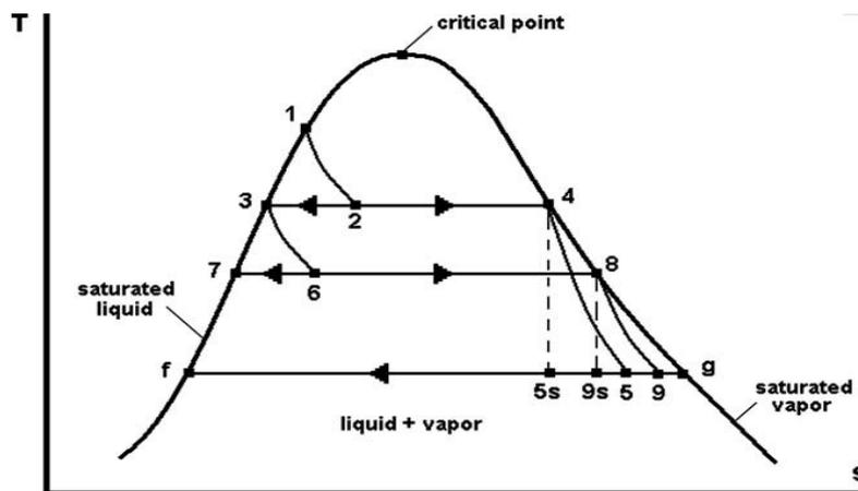
Figure 4 Temperature entropy diagram for the double flash plant
