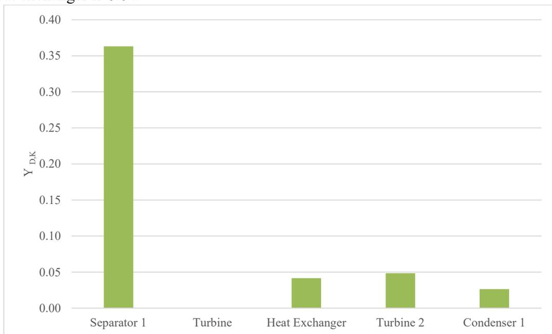
**Figure 13 Exergy destruction ratio for flash-binary plant**
