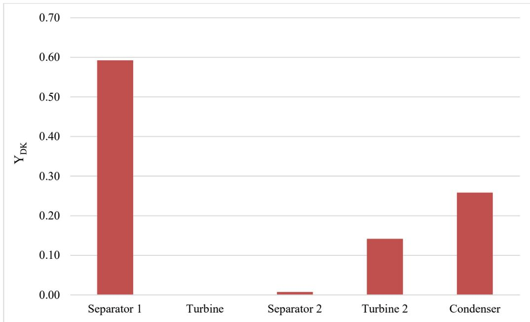
**Figure 12 Exergy destruction ratio for double flash plant**
