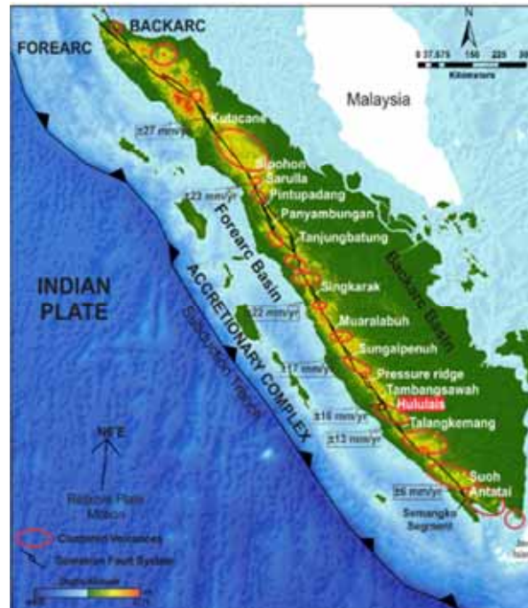
Figure 2.2 High-temperature geothermal prospect areas along the Sumatran Fault. Note the location of the Hululais geothermal field in the southern part of Sumatra Island (Nurseto et al., 2021).
