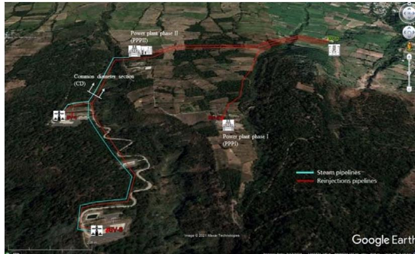
**Figure 6-27 Gathering system for Stage I & II utilising single flash units**
