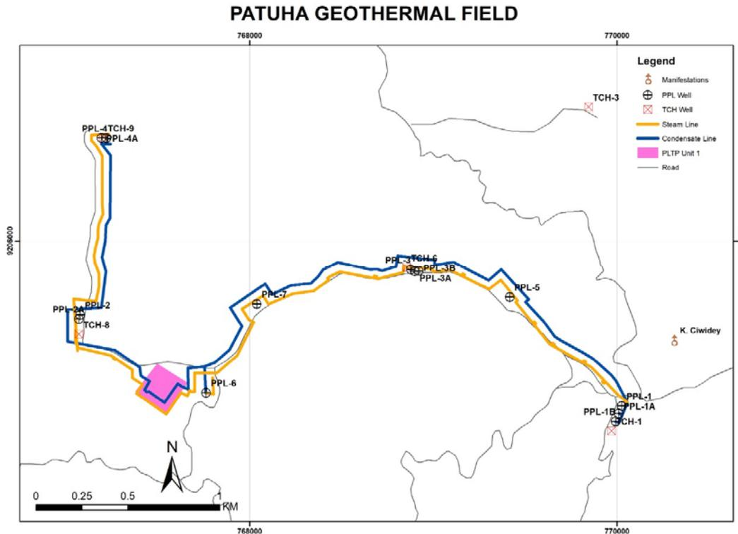
**Figure 1.3 - Location of the power plant and gathering system of the Patuha Geothermal Field**
