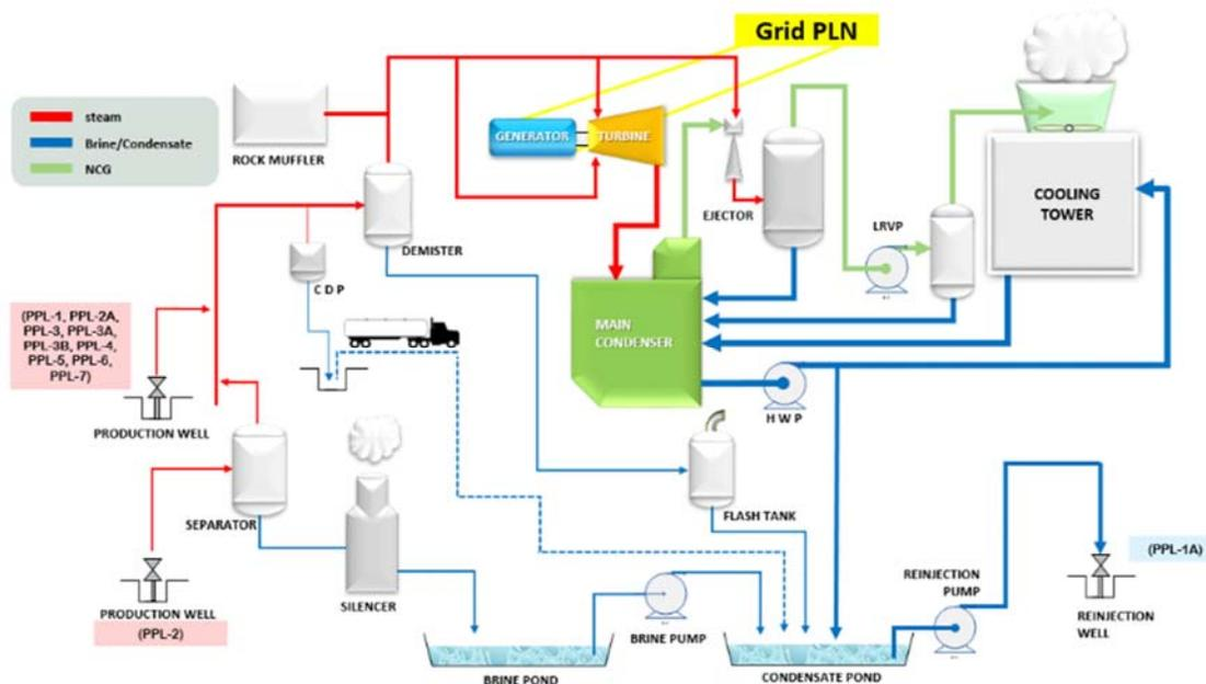
**Figure 1.4 - Process flow diagram of the Patuha Geothermal Field**
