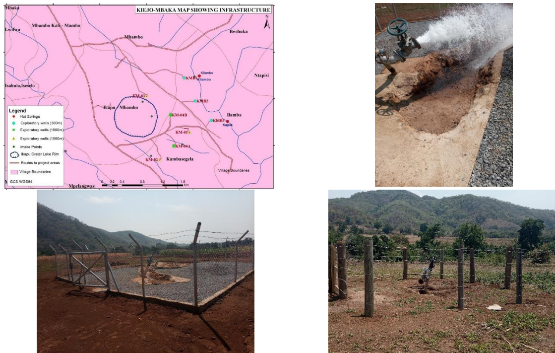
FIGURE 6: Simplified map showing well locations (top left) and drilled wells photos at Kiejo-Mbaka geothermal field
