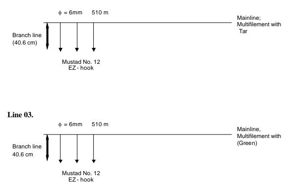
Figure 6: Gear parameters with the experimental longline gear module.
