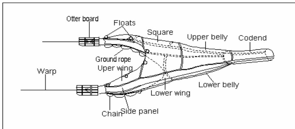
Figure 5: Diagram of different sections of a shrimp trawl net made of four panels.
