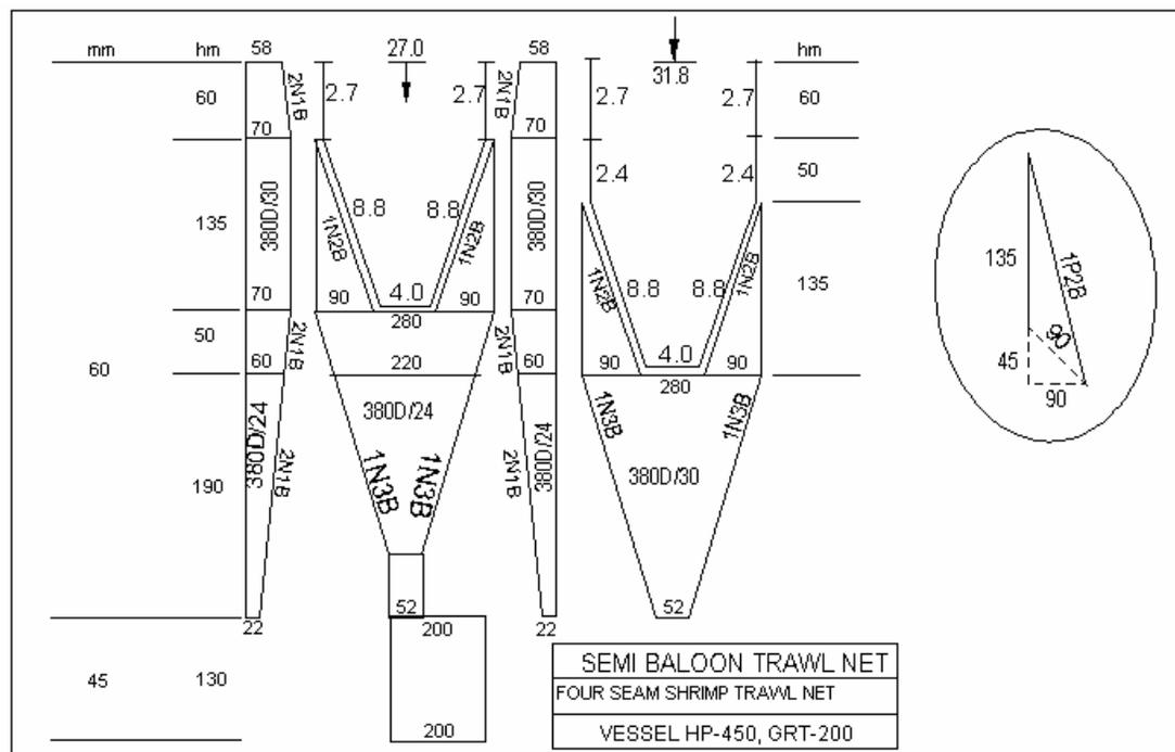
Figure 6: A drawing of trawl prototype used in Tanzania.
