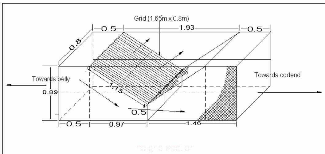
Figure 12: A diagram of the grid section designed and constructed in this study.
