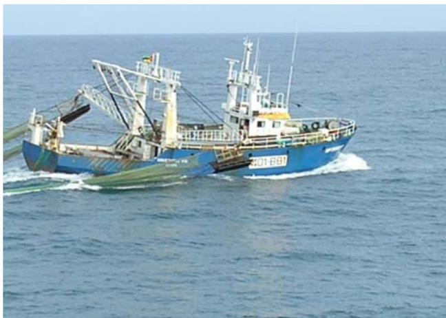
Figure 8: A Tanzanian shrimp trawler showing a double rig trawl.
