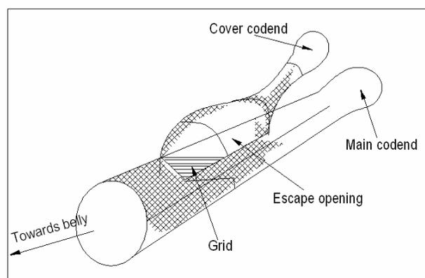
Figure 3: A diagram of cod end with over net
