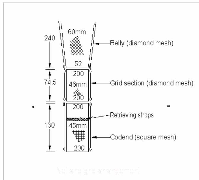
Figure 13: A diagram of grid and net arrangement (zippers).
