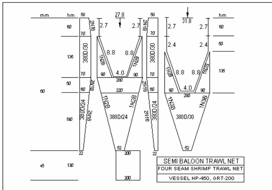
Figure 10: A drawing of trawl prototype used in study.
