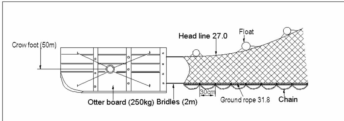
Figure 7: Diagram of trawl net wing and the trawl door arrangement used in Tanzania.
