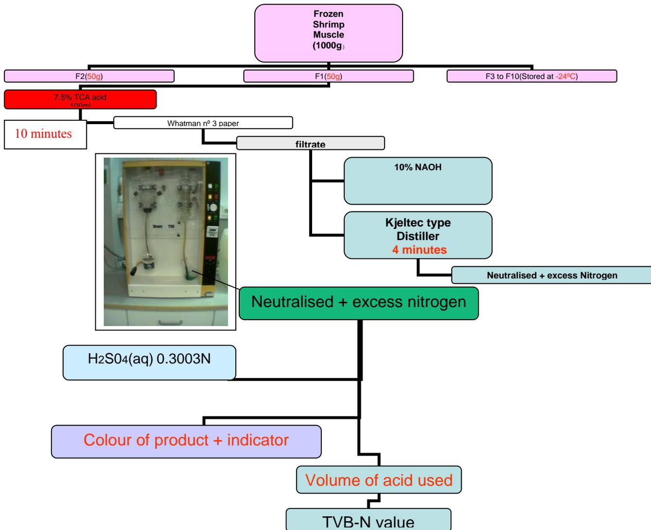
**Figure 20:** Flow diagrams for TVB-N analysis & Kjeltect type distiller in set.
