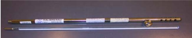
**Figure 12: Maximum reference thermometer.**
