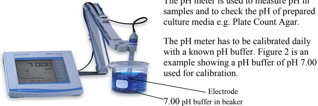
The pH meter is used to measure pH in samples and to check the pH of prepared culture media e.g. Plate Count Agar.
