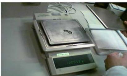
**Figure 4: Cleaning the balance.**
