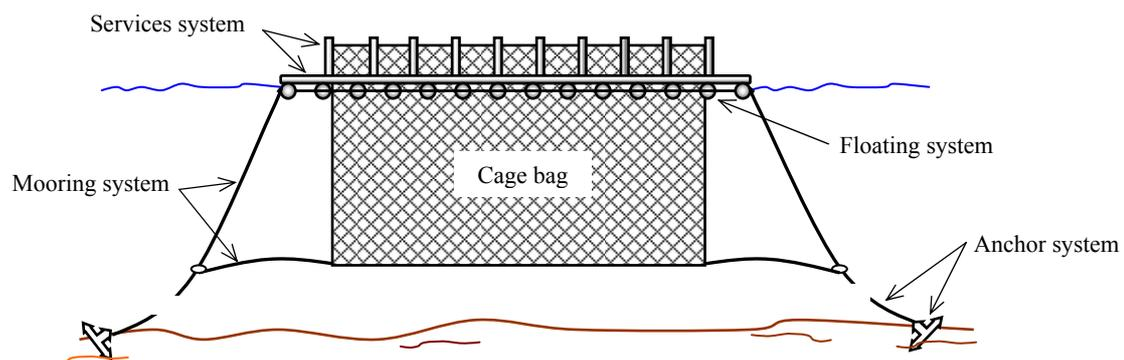
Figure 6: Principal components of the cage for farming.
