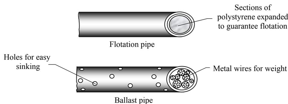
Figure 12: Details of the proposed flotation and ballast pipes made of high-density polyethylene (HDPE).
