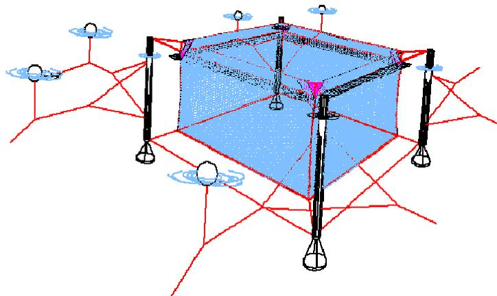
Figure 3: Anchor tensioned cages class (Loverich and Gace 1997).
