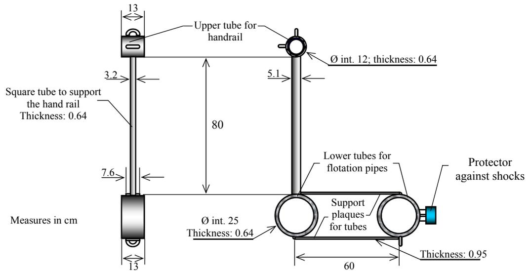
Figure 18: Parts and measures of the bracket.
