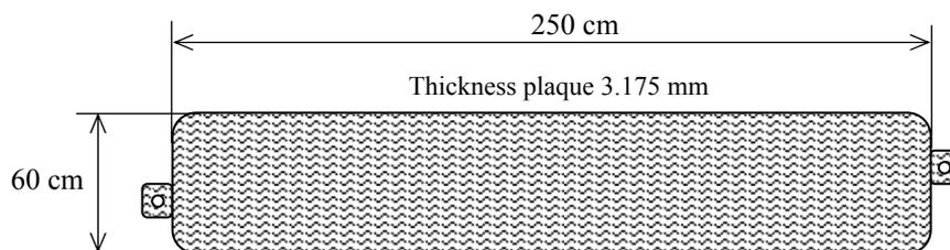
Figure 19: Approximate measurements of panels for the catwalk.
