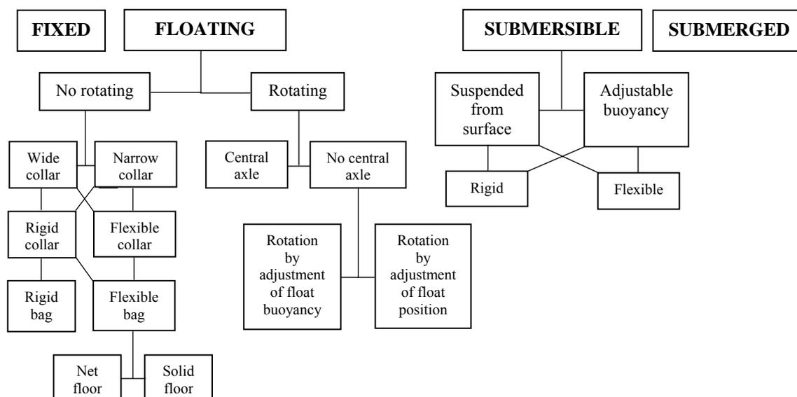
Figure 1: A classification system for cages by way of operating (Beveridge 1996).
