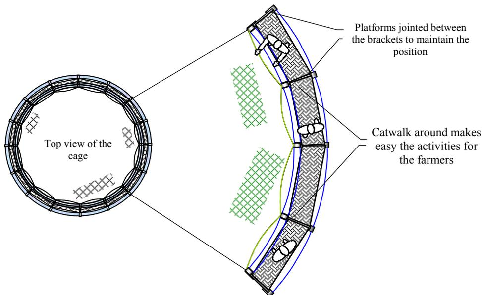
Figure 14: The catwalk around the cage will hold the brackets in its place and will facilitate feeding and maintenance.
