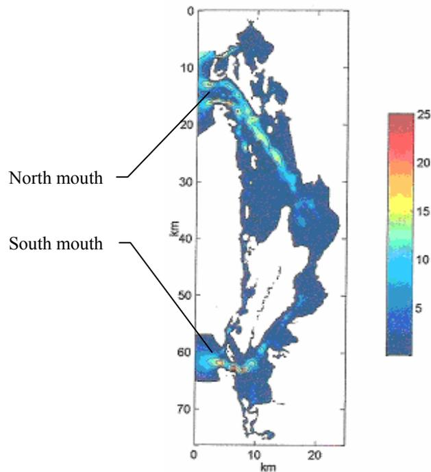
Figure 9: Bathymetry of the “Santa María La Reforma” Bay, Gulf of California (Serrano 2003).
