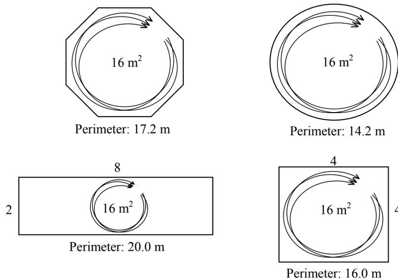
Figure 10: Perimeter lengths of different cage shapes for the same surface area and the circular swimming pattern of fish (modified from Beveridge 1996).
