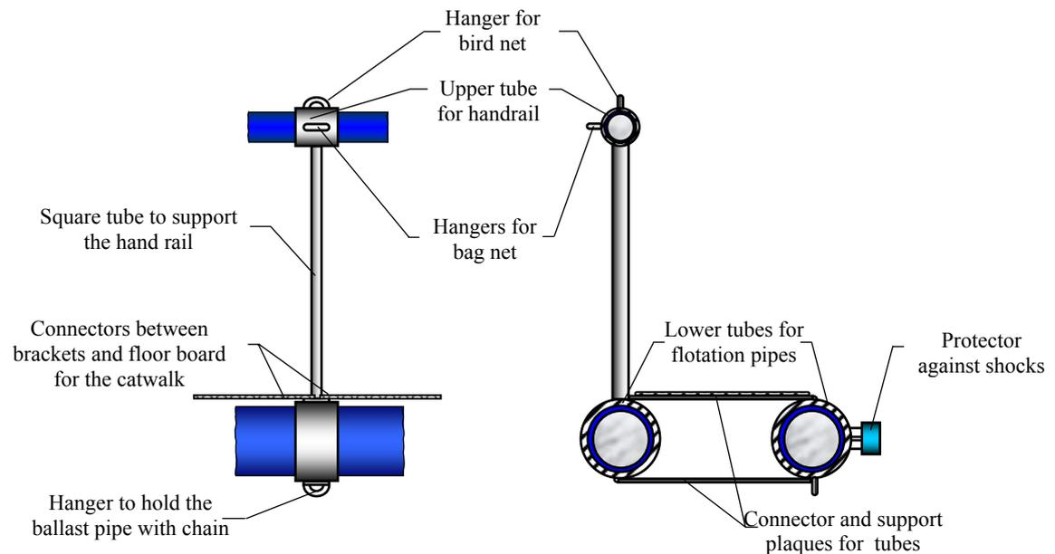
Figure 13: Brackets to hold the flotation and handrail pipes forming the structure of the cage and supporting the floorboards of the catwalk.
