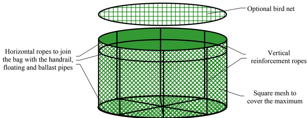
Figure 15: Cylinder cage bag with vertical and horizontal ropes for reinforcement and joints with the rings.
