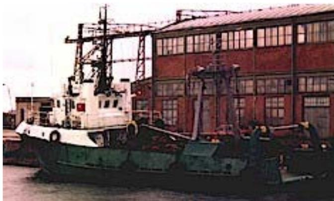
Figure 2: The main vessel type in the Baltic Sea is a small stern trawler - MRTK as show in this figure.
