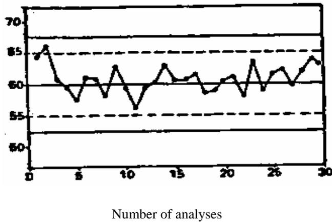
Figure 5: Control chart with warning and action limits in which results from 30 determinations have been recorded.
