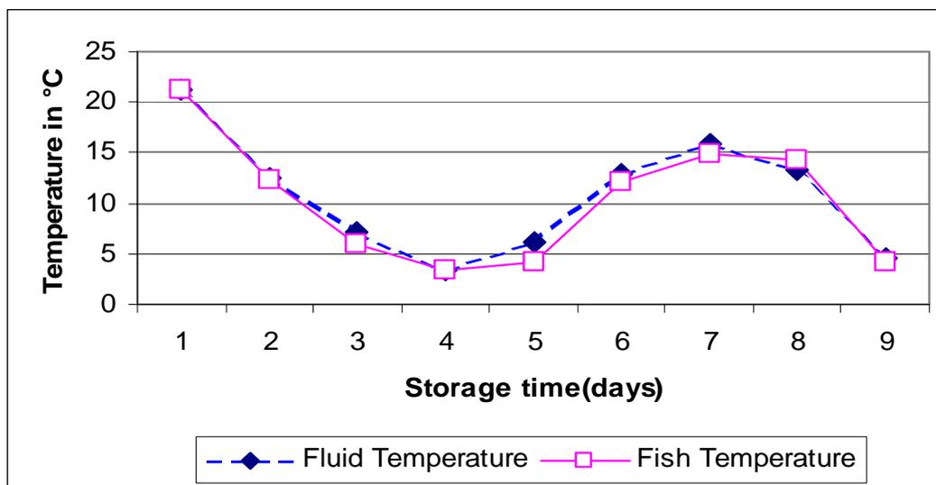
Figure 16: Core temperature of fish kept in ice at 25° room temperature. Measurements were taken daily.
