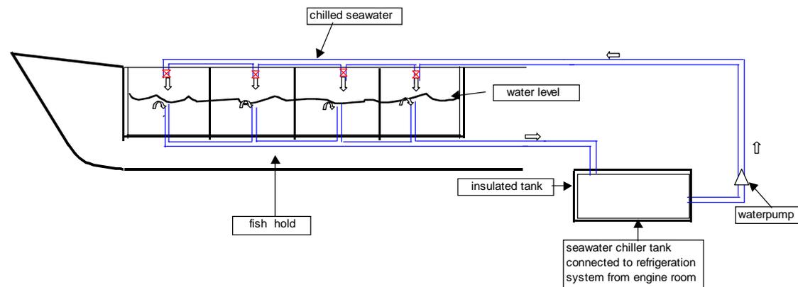
Figure 17: Proposed design of RSW system for a purse seiner.
