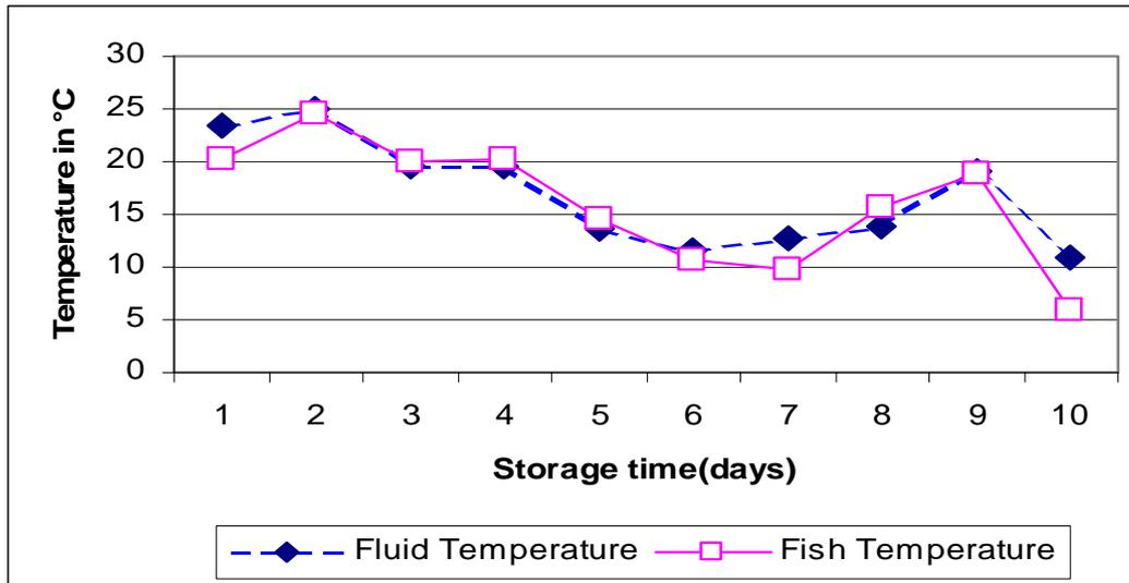
Figure 15: Core temperature herring kept in CSW at room temperature of 25°C. Measurements were taken daily.
