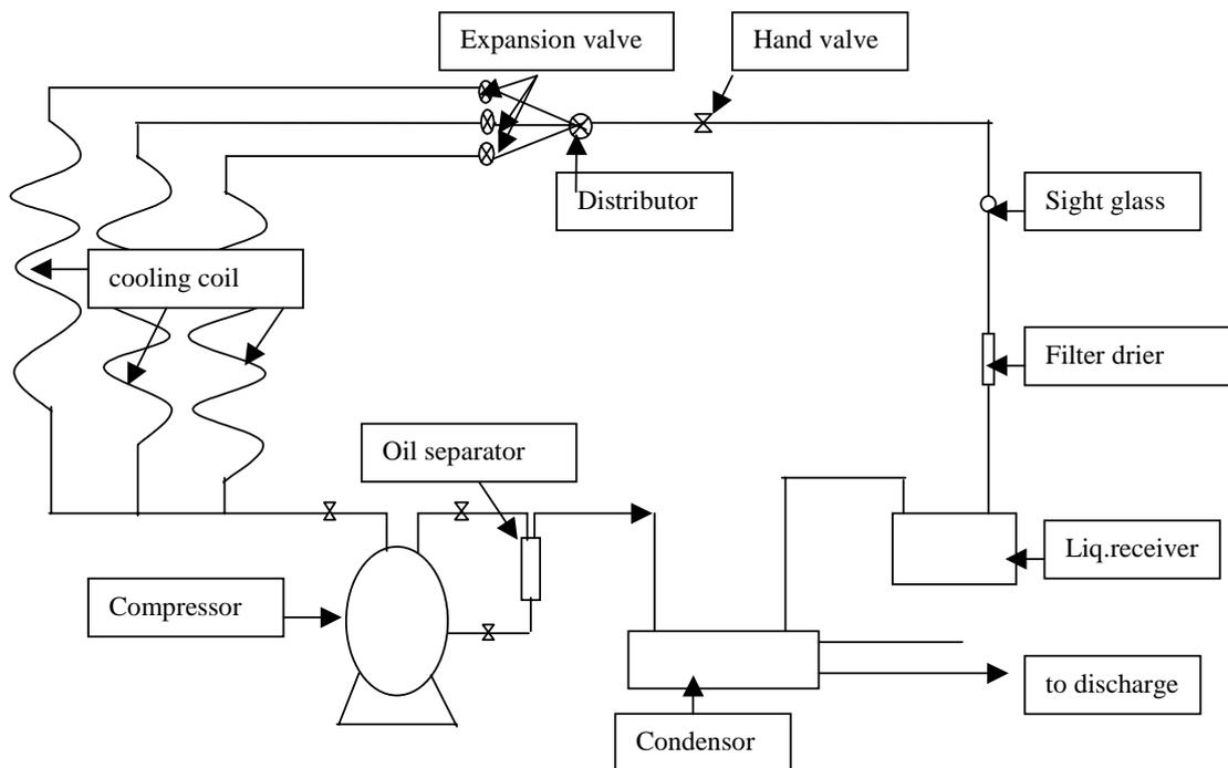
Figure 1: Refrigeration piping system layout installed in most existing fishing boats, especially trawlers, in Malaysia.
