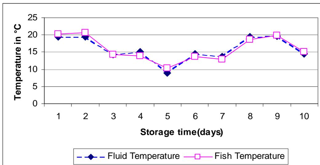
Figure 14: Core temperature of herring in liquid ice at 25°C taken daily.
