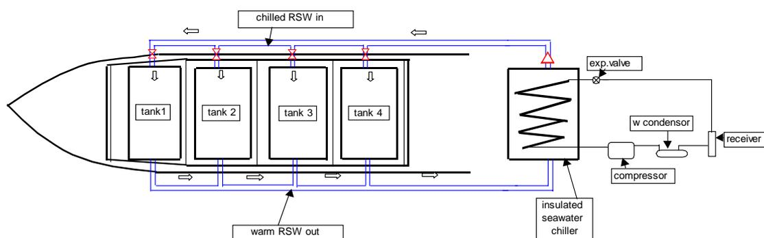
Figure 19: Proposed RSW system for a trawler.
