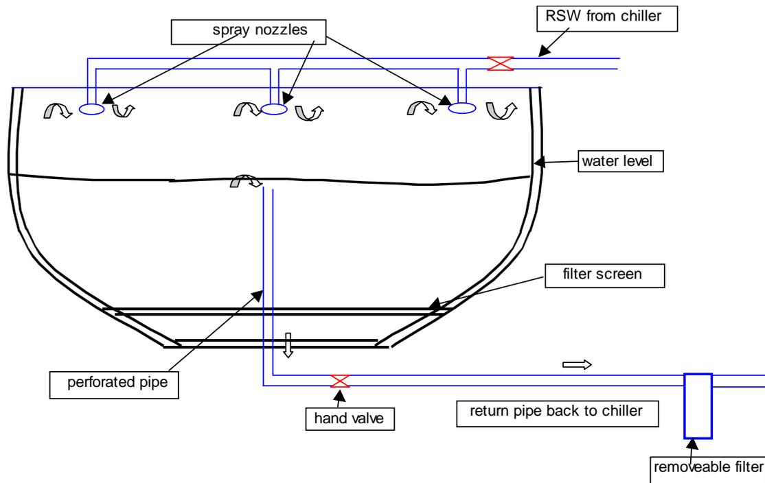
Figure 18: Cross section of RSW tank for a purse seiner.
