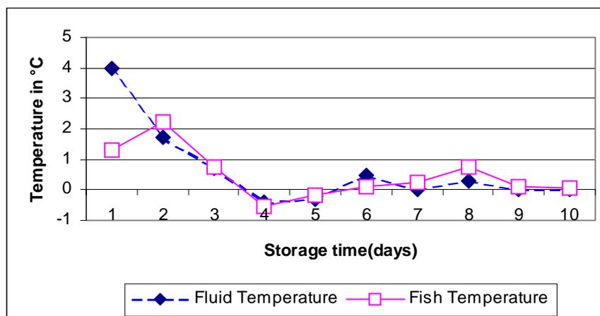
Figure 12: Core temperature of herring kept in CSW at  $2^{\circ}\text{C}$  taken daily.
