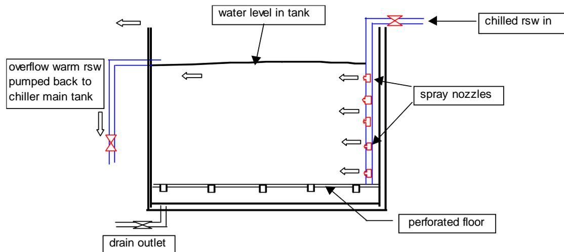
Figure 20: Cross section of RSW tank for trawler.
