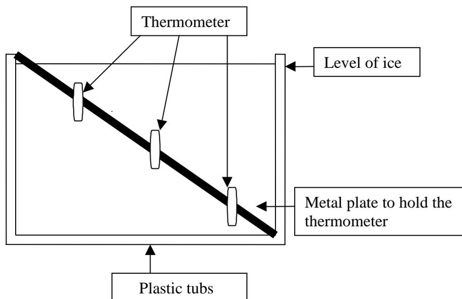
Figure 2: Location of the three onset thermometers in plastic tubs during ice melting trial to log the temperature.
