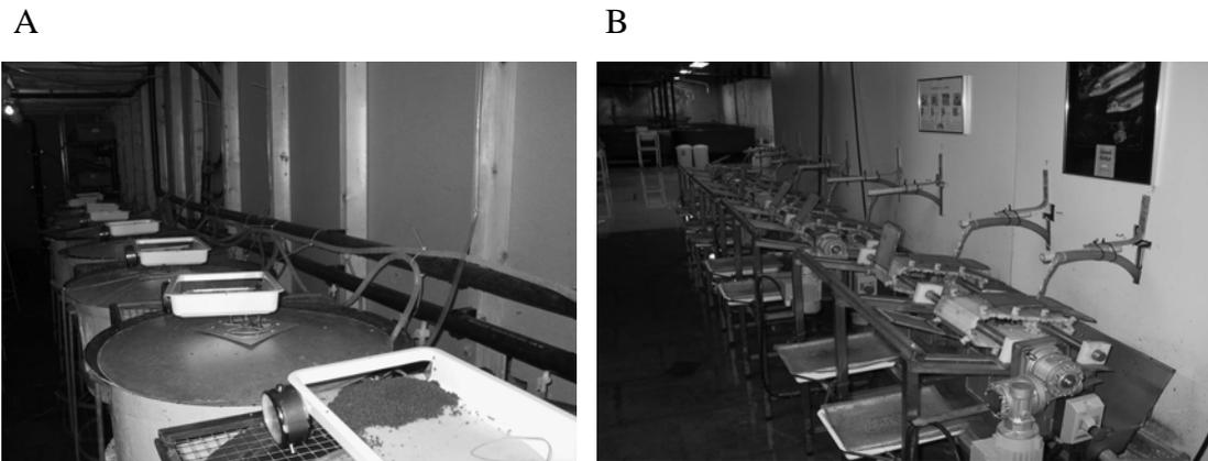
Figure 2: The experimental tanks with automatic feeding machines on top (A). The conveyer grid system collects faecal material from the tank (B).
