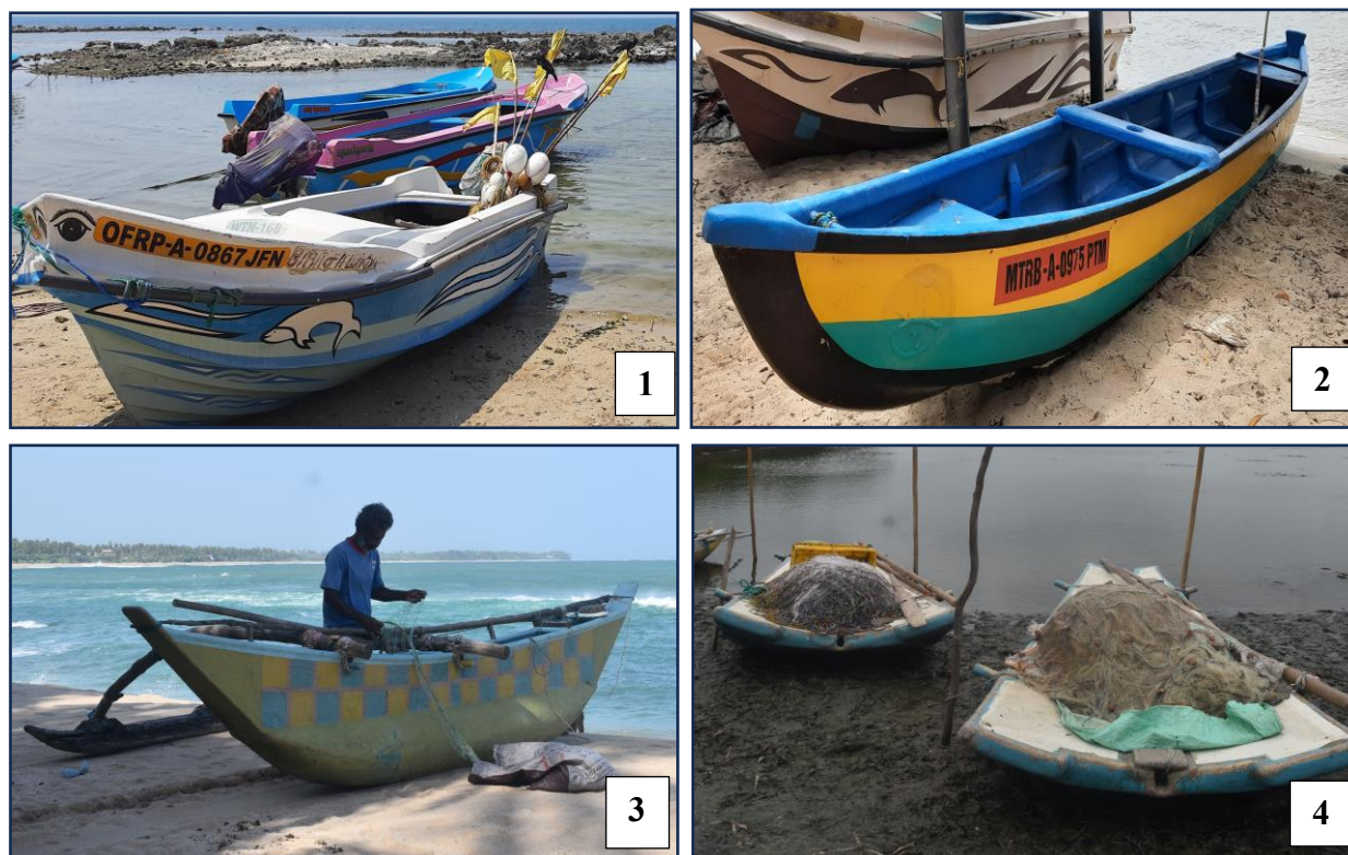
Figure 2: Small scale coastal fishing boats/craft used in coastal fishing operations. (1) OFRP-out-board engine fiberglass reinforced plastic boats, (2) MTRB-motorised (3) NTRB-non-motorised traditional boats.
