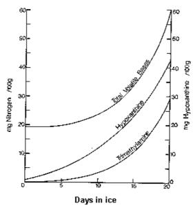
Figure 3: The changes in concentrations of TVB, Hx and TMA with the degree of spoilage of cod. (Connell 1990).
