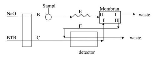
Figure 1: A schematic diagram of the Flow Injection/Gas Diffusion apparatus used for the determination of TVB-N.
