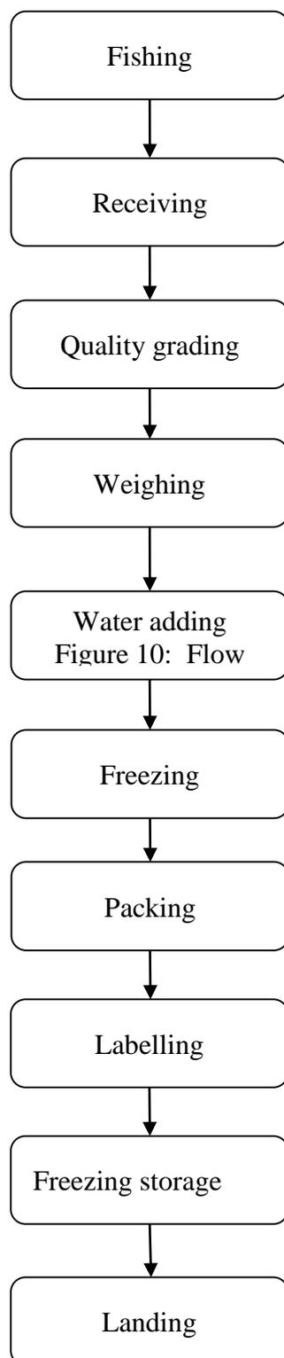
Figure 10: Flow chart for production of squid, frozen at sea.
