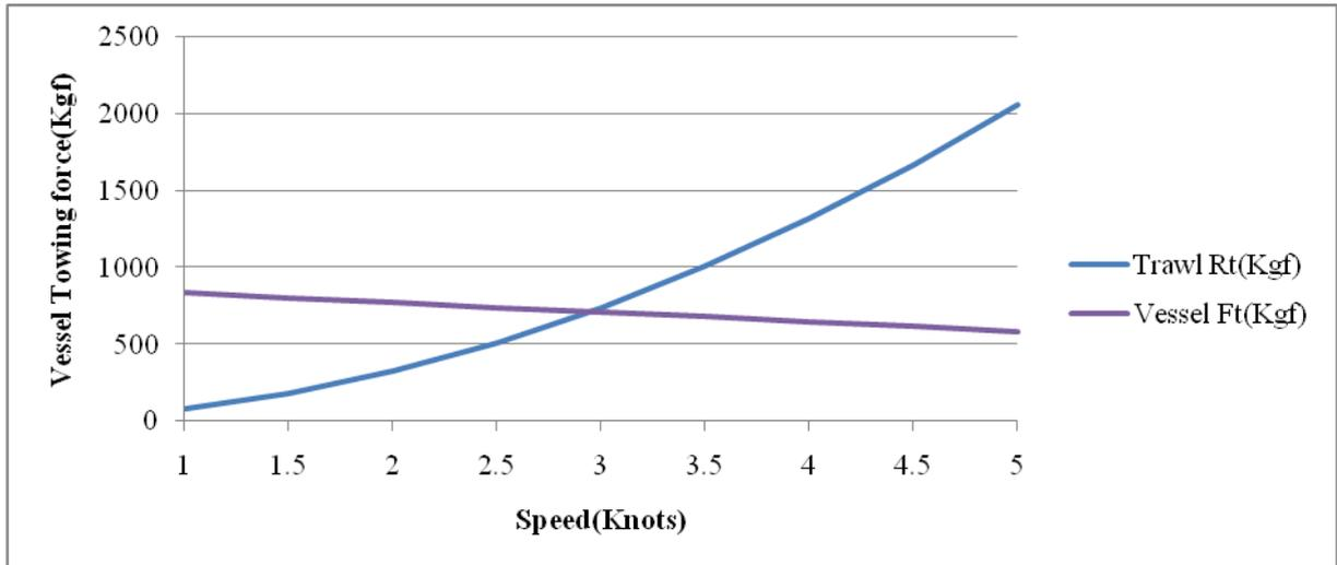
Figure 9: Comparison of vessel towing force (Kgf) and trawl resistance (Kgf) at 0.2 hanging ratio
