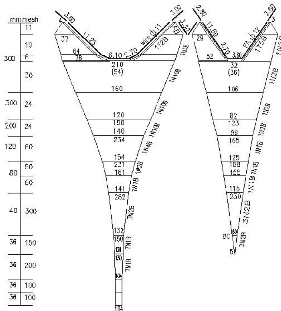
Figure 7: Prototype design of midwater pair trawl (FAO 1978). see details of specifications (Appendix 2)
