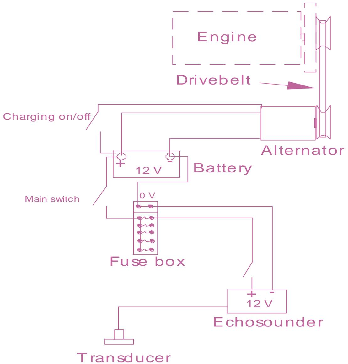
Figure 15: A basic arrangement showing echo sounder and DC connection
