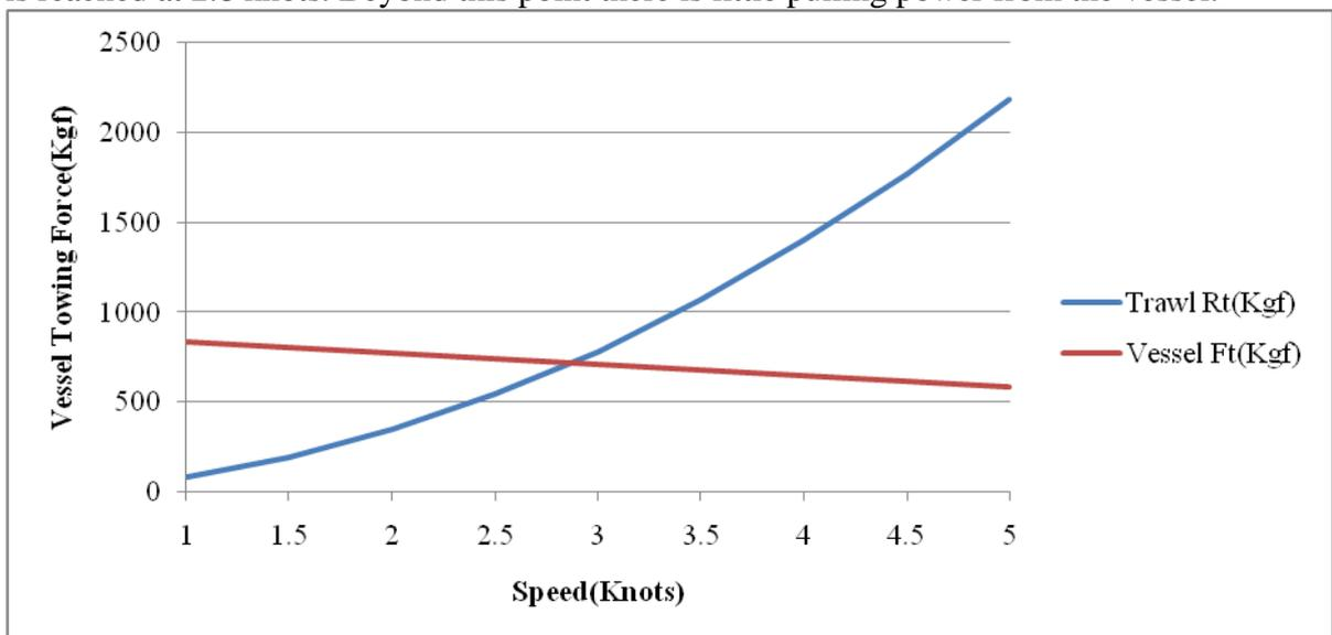
Figure 10: comparison of vessel towing force (Kgf) and trawl resistance (Kgf) at 0.3 hanging ratio
