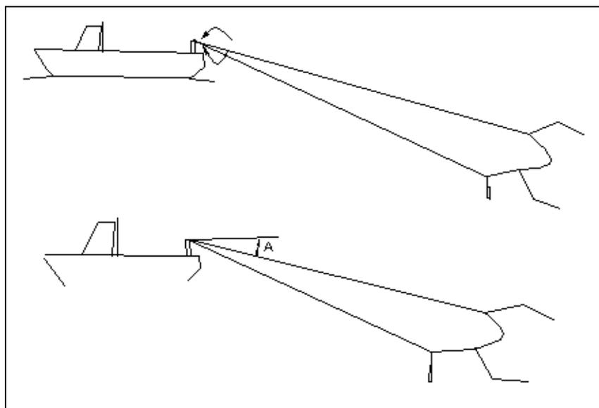
Figure 16: Warp angle A during trawling estimated with a protractor or string.
