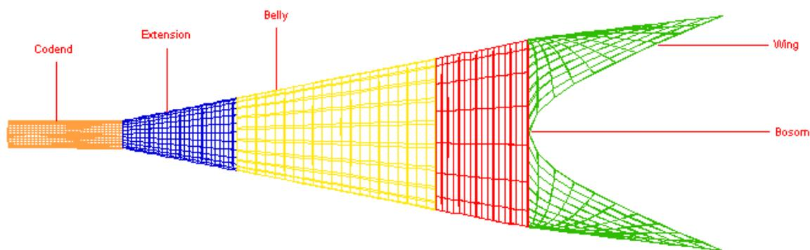
Figure 6: Main part of the midwater trawl net
