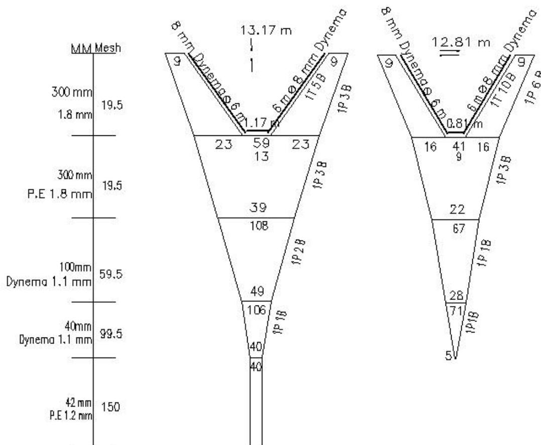
Figure 8: New design for a midwater pair trawl. See details of specifications in Appendix 3.
