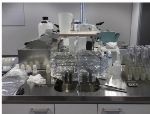
Figure 1: Experiment set up for cleaning and swabbing of test surfaces. From right to left: stopwatch, glass tubes with fouled coupons, spray bottles (water, detergent, sanitizer), rack with to-be-cleaned coupons (triplicate), cleaned coupons to be swabbed and bottles for swab heads.
