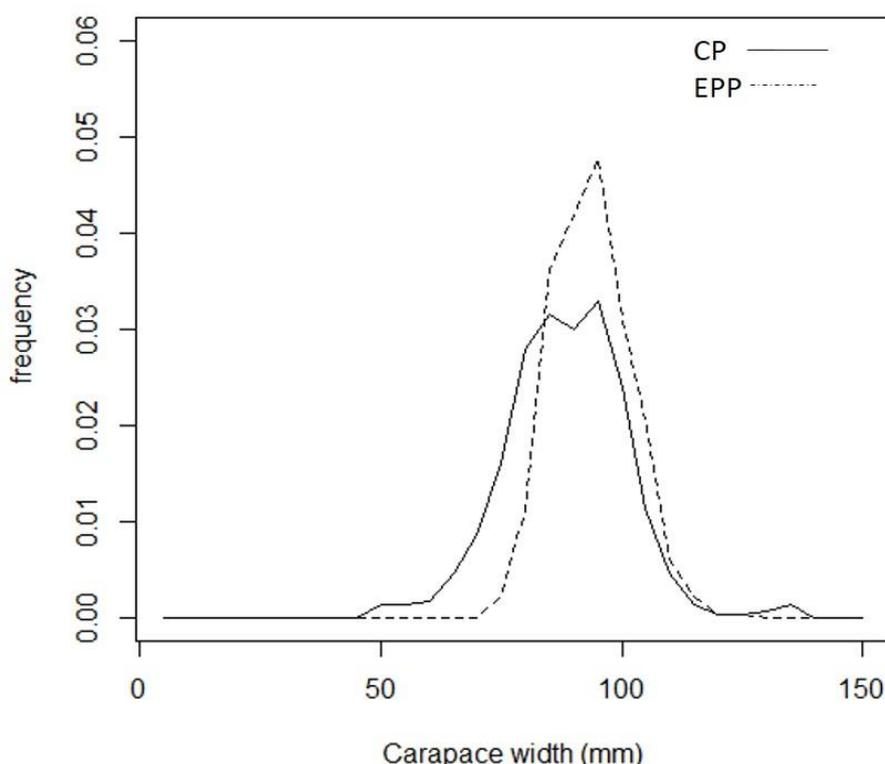
Figure 12. Size frequency distribution (carapace width) caught in the two different blue crab pot CP (Creole pot) and EPP (Escape panel pot).
