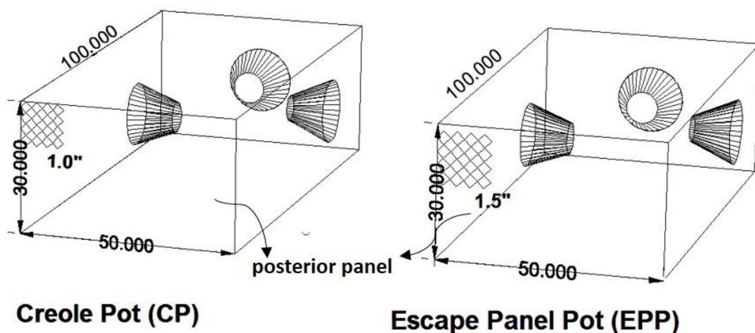
Figure 6: Two different pots, Creole pot (CP) and Escape panel pot (EPP) used in the experiment. Mesh size indicated in inches.
