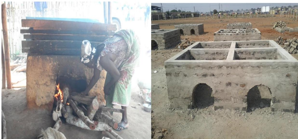
Figure 3: Types of Chorkor smokers. To the left: A Single mud base Chorkor Smoker with stackable wooden trays; To the right: A double cement base Chorkor smoker.
