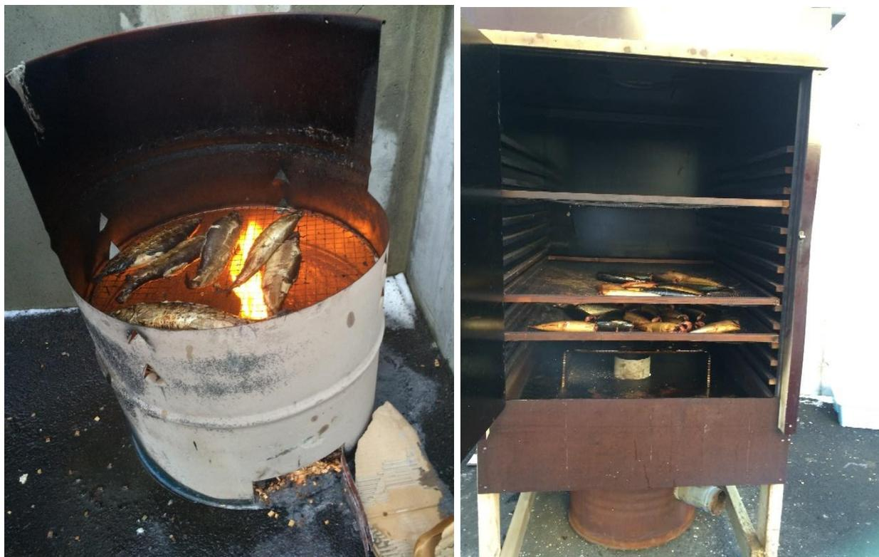
Figure 5: The smoking equipment used in the study. To left: Open fire smoking kiln; To right: Smoking cabin designed by MATIS.
