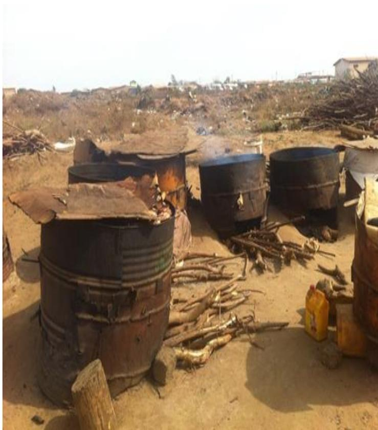
Figure 4: Cylindrical drum ovens.
