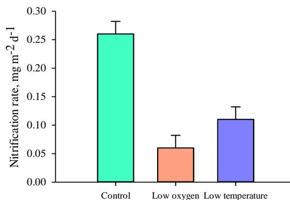
Figure 11: The average nitrification rate between the groups (The bars show standard error).
