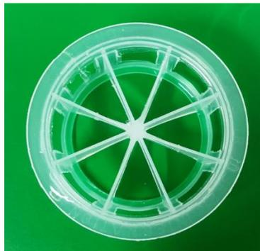
Figure 4: Biofilter media. The plastic ring with SSA 236.25 m<sup>-2</sup> m<sup>3</sup>.
