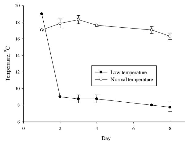
Figure 9: The temperature in the control biofilters and in the biofilters that were cooled down. The vertical bars show standard deviation.
