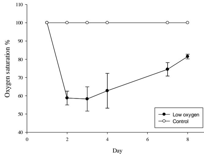
Figure 8: The oxygen levels in the control biofilters and in the biofilters where aeration was suspended (The vertical bars show standard deviation).
