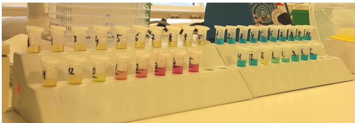
Figure 6: Samples of TAN and NO<sub>2</sub> with reagents prepared for reading on spectrophotometer.
