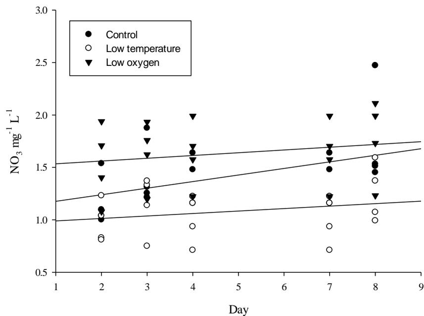
Figure 14: Nitrate concentration during the experiment. The lines show the linear relationship between nitrate concentration over time. The parameters of the equation are given in Table 5.
