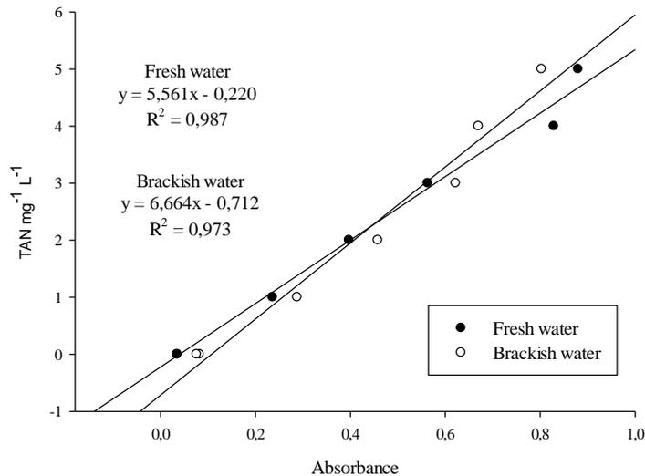
Figure 7: Comparable analysis of two TAN standard curves based on fresh and brackish water.
