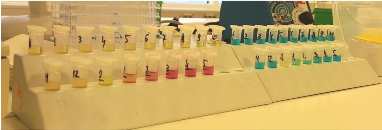
Figure 6: Samples of TAN and NO<sub>2</sub> with reagents prepared for reading on spectrophotometer.
