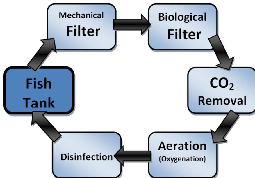
Figure 1: Schematic diagram of RAS.
