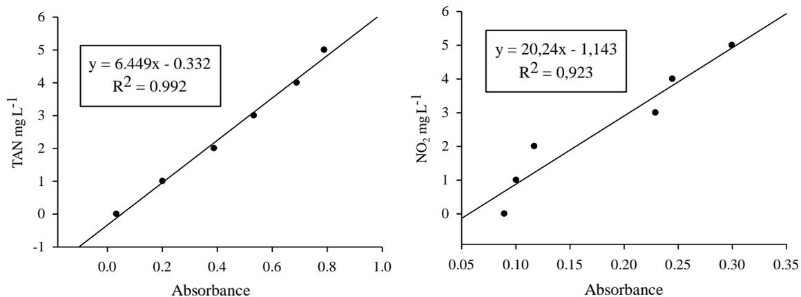
Figure 5: Examples of standard curves for TAN and  $\text{NO}_2$ .
