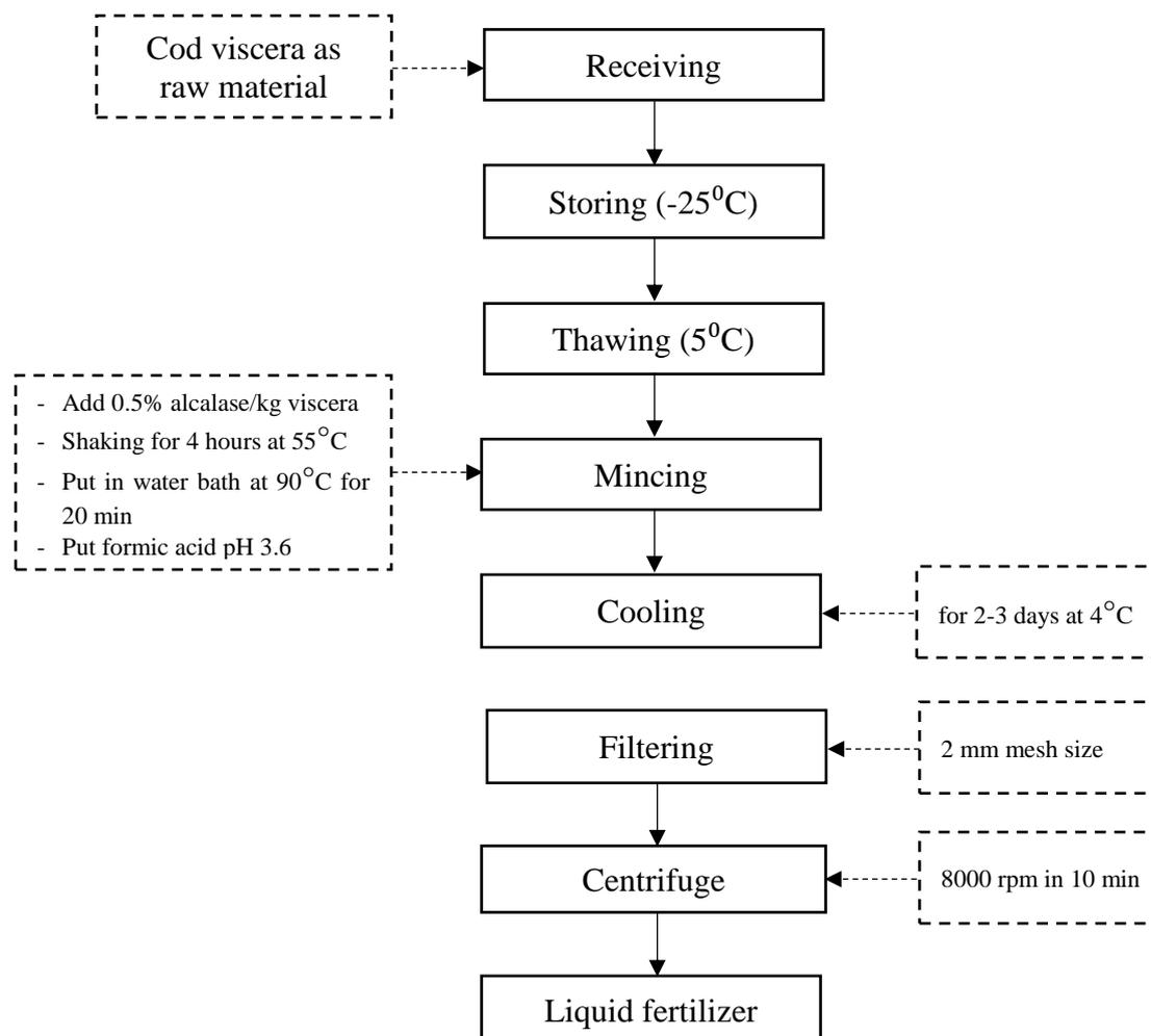
**Figure 5. Flow chart of industrial enzyme treatment in liquid fish silage production.**
