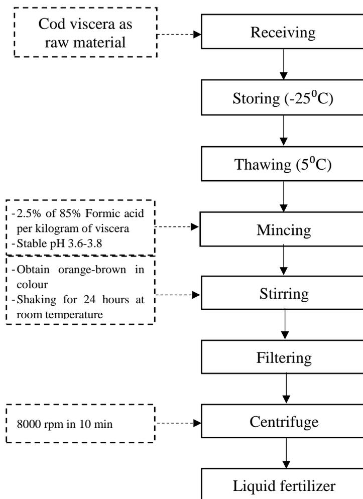
**Figure 4. Flow chart of natural enzymes treatment in liquid fish silage production.**
