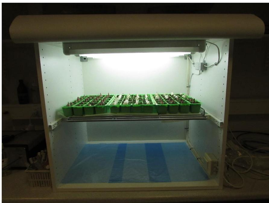
**Figure 6. A chamber with fluorescent light used for planting onion and garlic plants for the experiment.**
