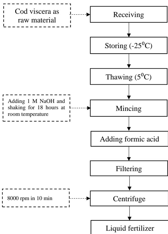
**Figure 3. Flow chart of alkali treatment in liquid fish silage production.**
