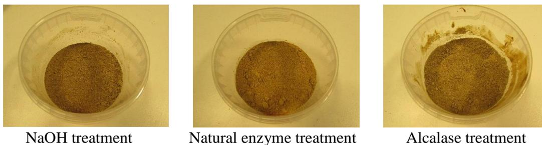
**Figure 12. Final product of solid/dried fish silage using NaOH treatment, natural enzyme treatment and alcalase treatment.**
