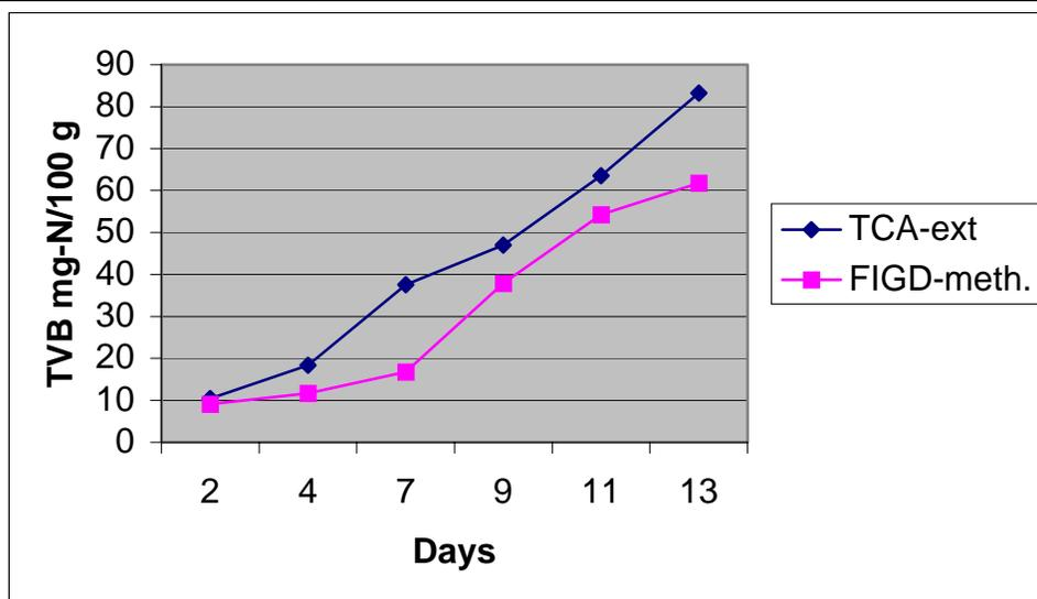
Figure 5. TVB analytical methods (TCA-extract , FIGD) used to determine freshness of herring that was stored at 0°C for up to 13 days.
