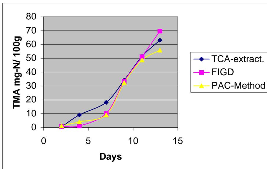
**Figure 9. Comparison of TMA results of herring stored at 0°C for up to 13 days by using TCA-extract, FIGD and Picric acid methods.**
