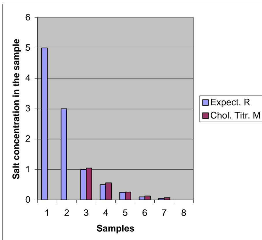
Figure 3. Results of chloride titrator method and expected values in salted water solutions.
