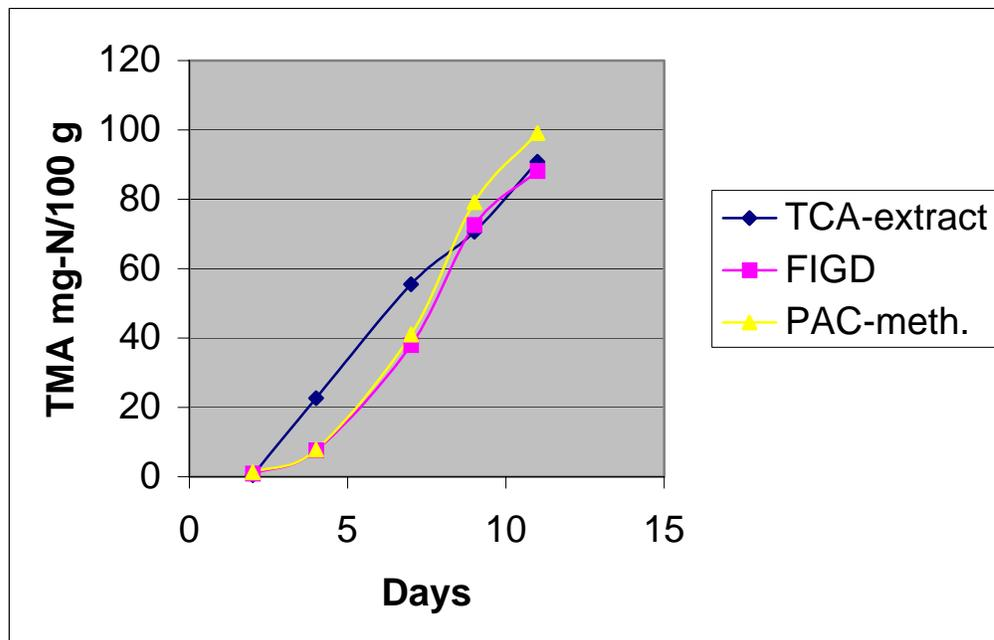
**Figure 10.** Comparison of TMA results of herring stored at 5°C for up to 13 days by using TCA-extract, FIGD and Picric acid methods.
