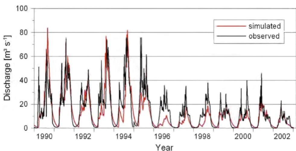
**Fig. 10.** Simulated and observed discharge of the River Kharaa near Darkhan (HBV-D Model) (Source: MOMO, 2009).
