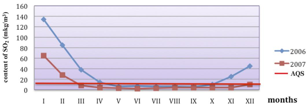
**Fig. 9.** Emissions of SO<sub>2</sub> based on data from Institute of Meteorology (2006, 2007).
