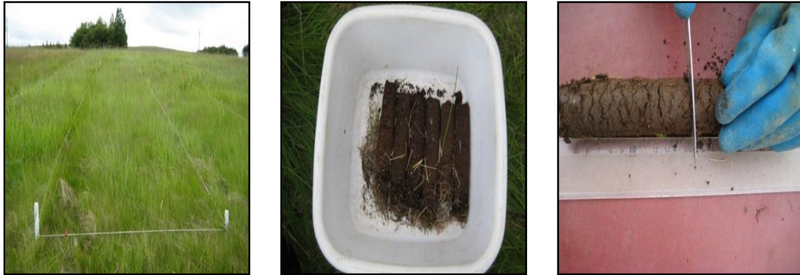
Fig. 4. The experimental field at Sámstaðir where subplots were bordered by rope (left). Soil samples from a subplot (middle). Cutting process of soil sample (right).
