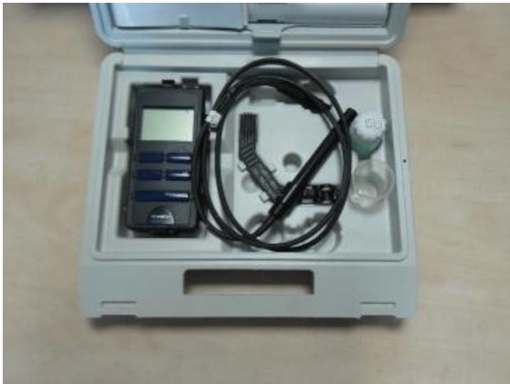
Figure 6. Conductivity meter used in this study (type: Cond 315i SET) produced by the German company Wissenschaftlich-Technische Werkstätten GmbH (WTW).
