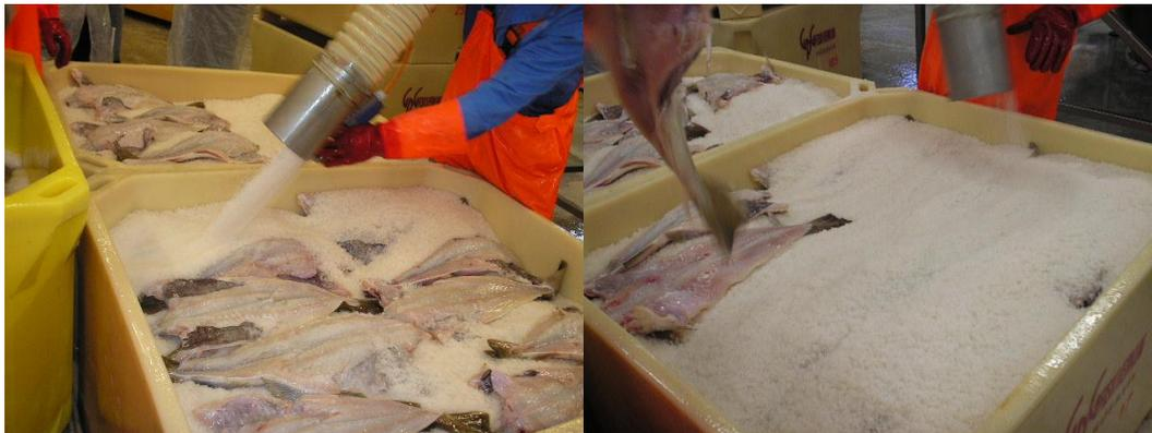
**Figure 9: Modern method of heavy dry salting in plastic containers after brining for 2-3 days. An improved method used for salt curing of “bacalao” in the western world.**
