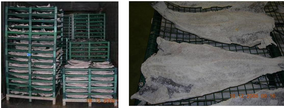
**Figure 15: Dried salted product on trolleys in a drying chamber.**
