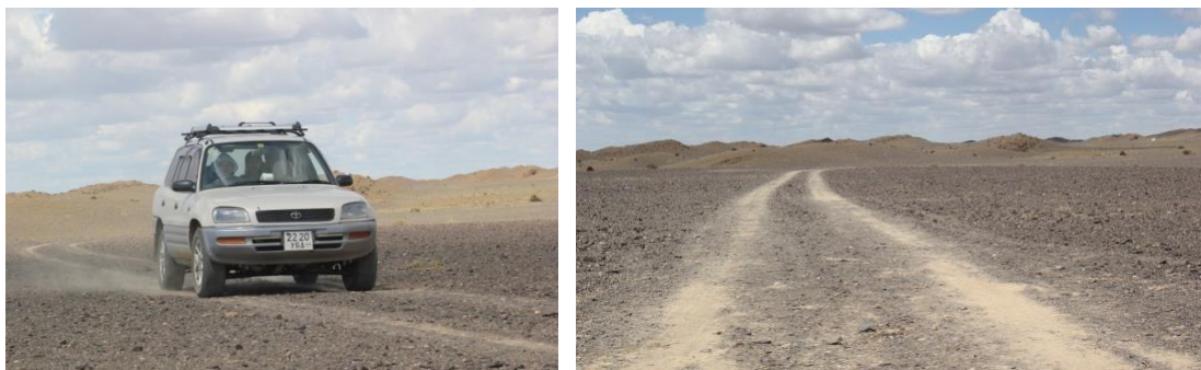
Figure 4. The off-road track simulation experiment. A 100-m stretch was driven 50 times to simulate the effect of typical off-road driving in southern Mongolia.
