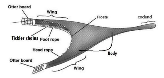
Figure 6. A bottom otter-trawl is a cone-shaped net comprising of a body which is closed by a codend and with adjacent wings spreading forward from the opening. The otter-trawl is kept open by two otter boards. Modified from Willems (2016 and references therein).
