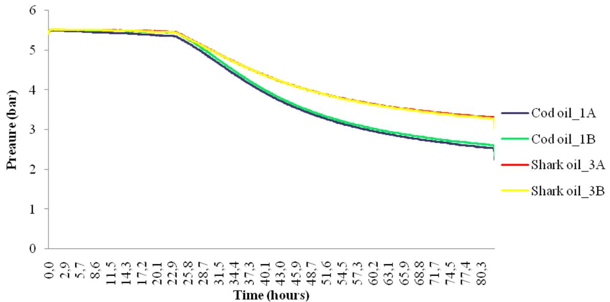
Figure 1: Induction period results from cod and shark liver oils.
