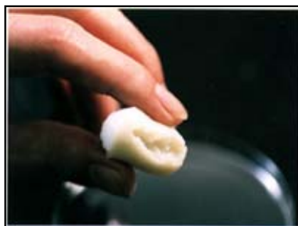
Figure 7: Folding test used for measuring the gel strength of cooked FPI gel.
