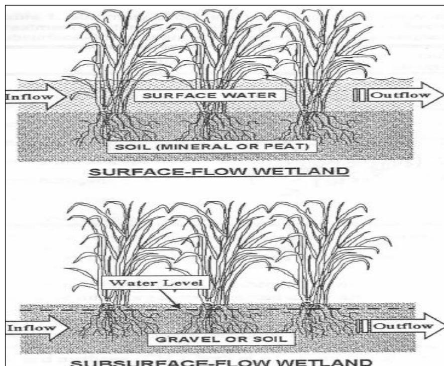
Figure 2: Diagram of surface-flow and subsurface-flow wetlands (DeBusk 1999).
