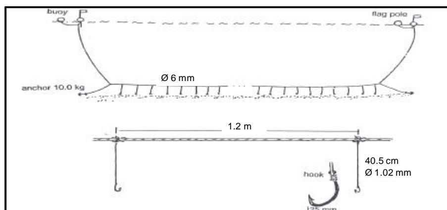
Figure 7: The whole view of a bottom set longline and hooking space. A mainline with a branch line carrying 500 hooks is set on the bottom by buoy and anchor (Hameed and Boopendranath 2000).
