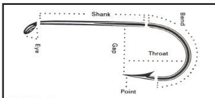
Figure 4: Basic parts of a J hook made of steel, coated with different metals (Bjordal and Løkkeborg 1996).
