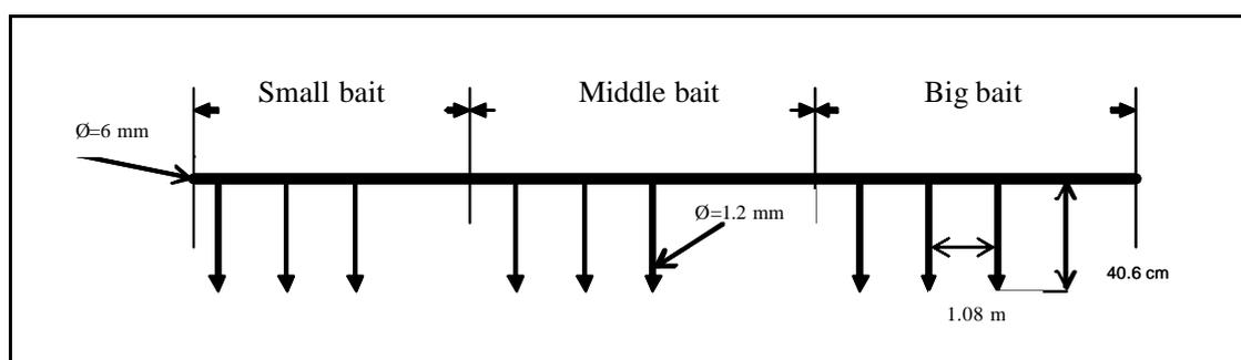
Figure 12: Longline arrangement for the experiment. Three lines with the bait sizes small (15 g), medium (25 g) and big were set in one skate.
