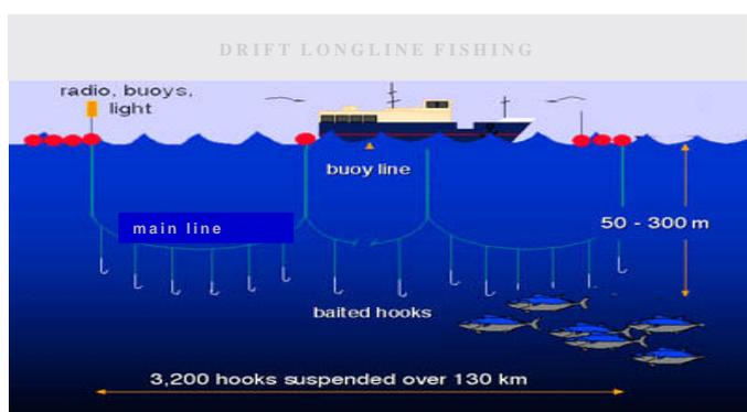
Figure 8: Drift longline set in a certain water depth by buoys is applied to catch fish migrating in mid-water (Birds Australia 2006).
