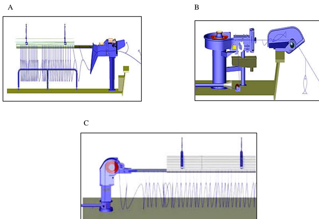
Figure 10: Different parts of an auto longline system. A) Baiting and Shooting, B) Hauling and C) Handling line (The three pictures are copied from Mustad Longline A.S 2006).
