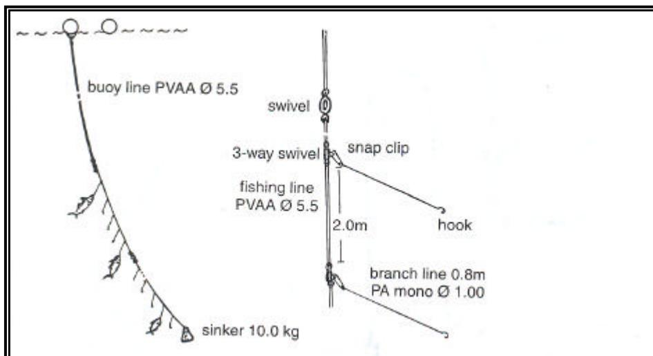
Figure 9: Vertical longline set vertically by buoy and anchor to catch fish migrating across a vertical range and connecting the branch lines to the mainline (Hameed and Boopendranath 2000).
